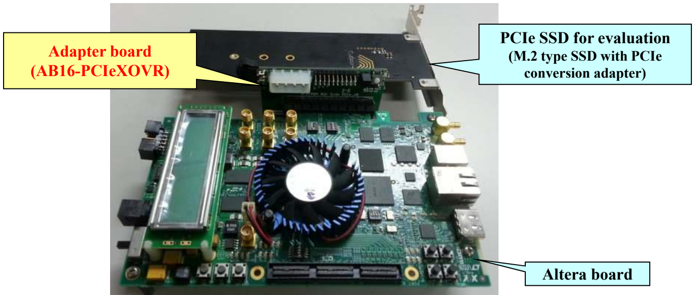
IP-Core evaluation environment using ArriaV GX Starter Kit
