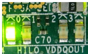
Figure 2-13 LED status after program configuration file and FAT32-IP initialization complete
