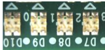
Figure 2-12 4-bit LED Status for user output
