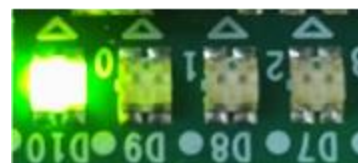
Figure 2-13 LED status after program configuration file and FAT32-IP initialization complete
