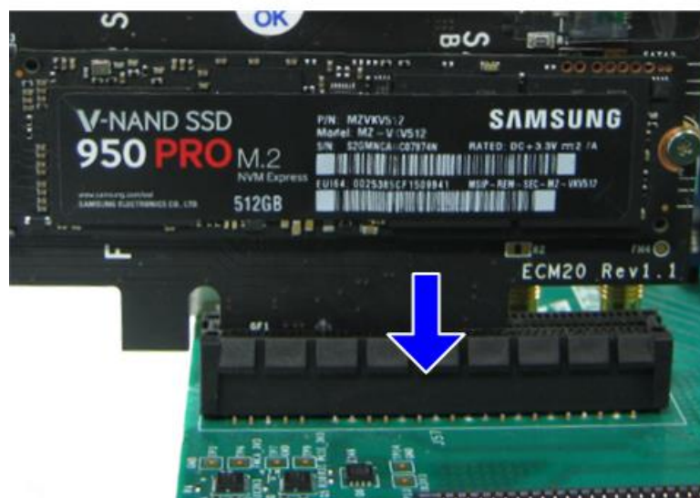
Figure 2-5 NVMe PCIe SSD connection on FPGA board
