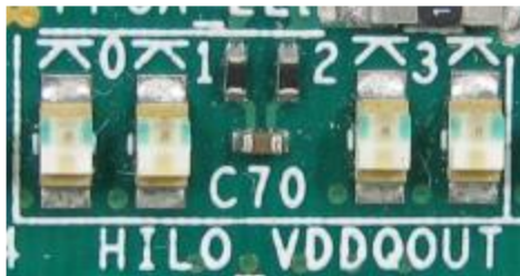
Figure 2-12 4-bit LED Status for user output
