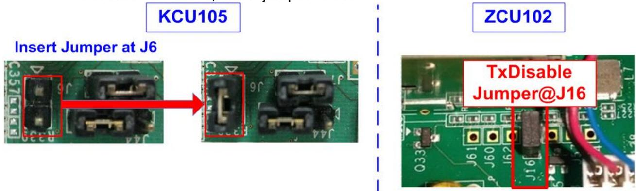
Figure 2-1 Insert jumper to enable SFP+ on KCU105/ZCU102
