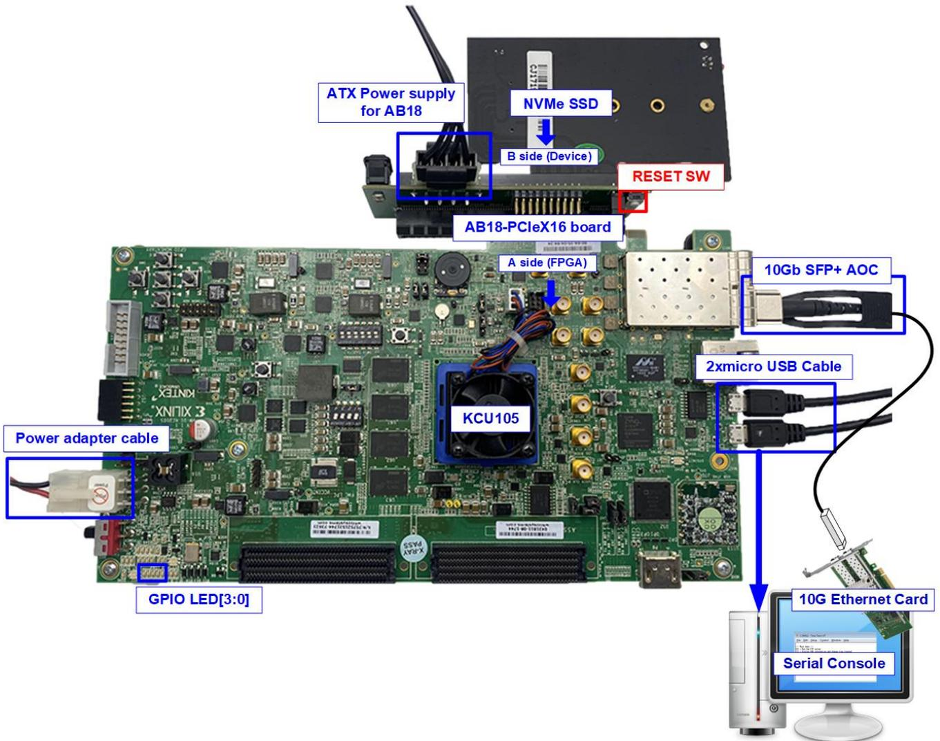
Figure 1-1 FTP Server demo on KCU105 with AB18
