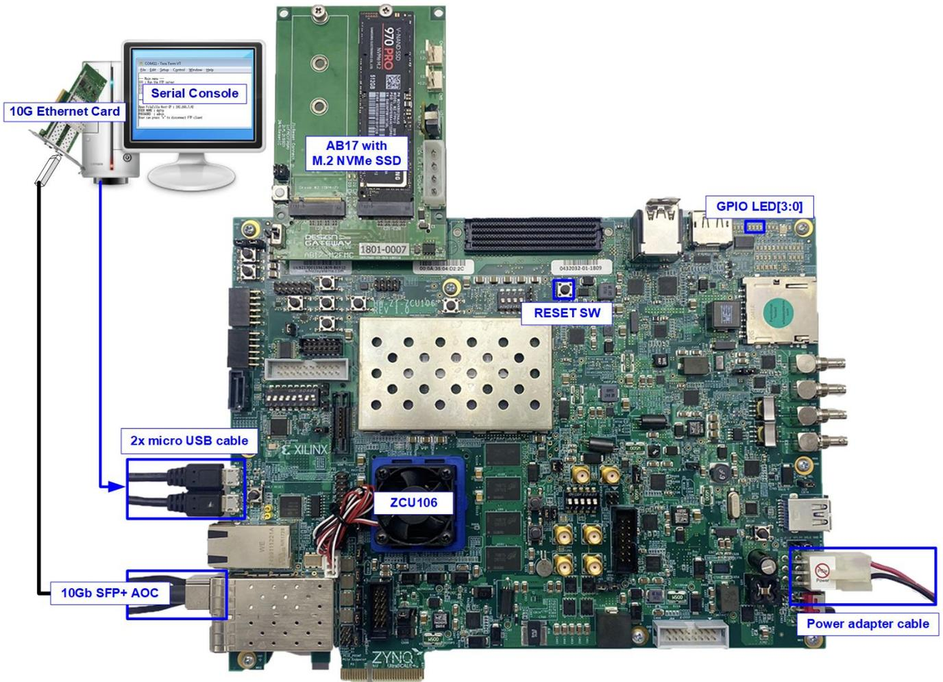
Figure 1-2 FTP Server demo on ZCU106 with AB17
