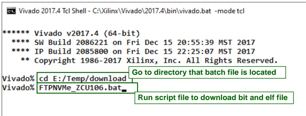
Figure 2-10 Command script to download demo file on Vivado TCL shell
