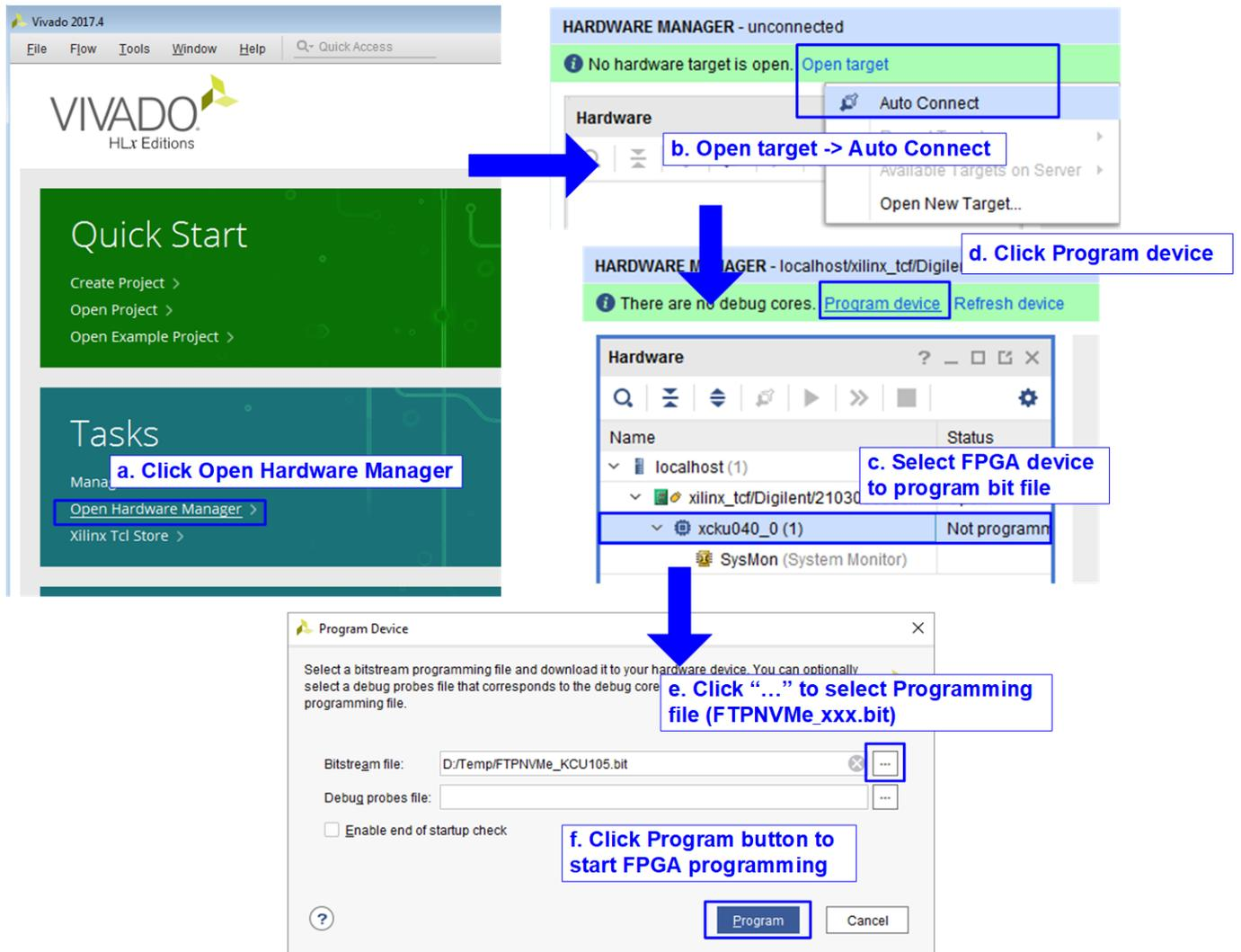
Figure 2-9 Program FPGA by using Vivado
