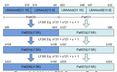
Figure 2-5 256-bit LFSR Pattern in TestGen
