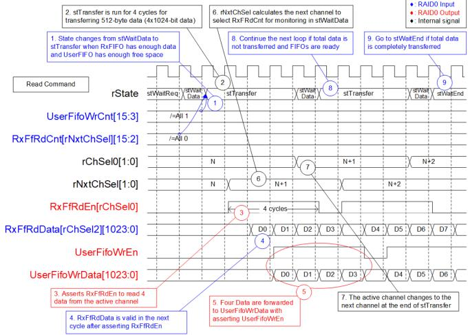
Figure 2-10 Raid0x2 timing diagram in Read command
