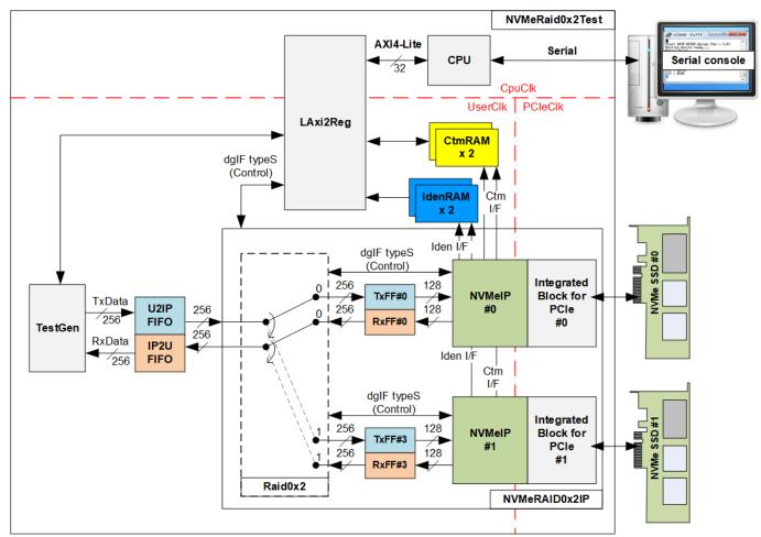
Figure 2-1 RAID0x2 demo system by using NVMe-IP
