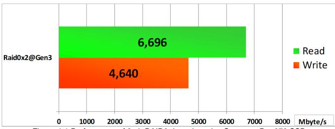
Figure 4-1 Performance of 2-ch RAID0 demo by using Samsung Pro 970 SSD
