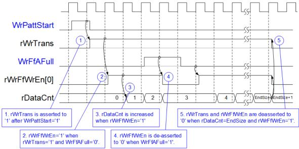
Figure 2-6 Timing diagram of Write operation in TestGen
