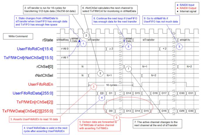
Figure 2-9 Raid0x2 timing diagram in Write command
