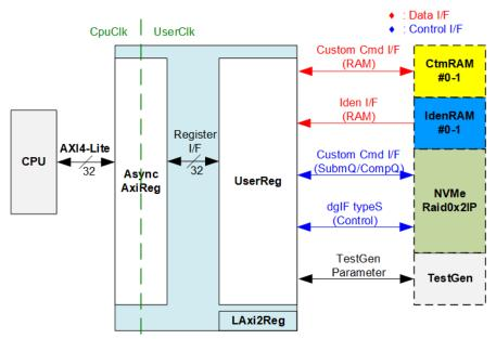
Figure 2-11 CPU and peripherals hardware
