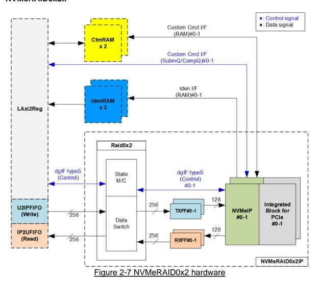
Figure 2-7 shows the example to interface NVMeRAID0x2 in the reference design. The user interface of NVMeRAID0x2 consists of control interface and data interface. The control interface receives the command and the parameters from custom command interface or dgIF typeS, depending on the command. Custom command interface is used when operating SMART command or Flush command.
