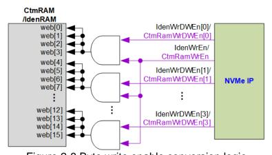
Figure 2-8 Byte write enable conversion logic
