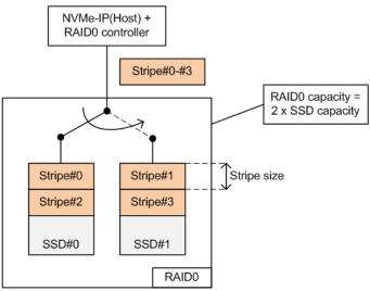
Figure 1-1 RAID0 by 2 SSDs data format
