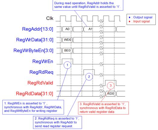
Figure 2-13 Register interface timing diagram
