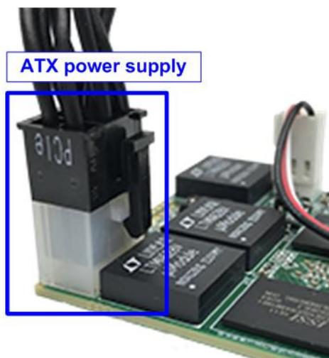
Figure 2-1 ATX power supply connected to FPGA
