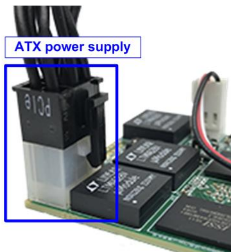
Figure 2-1 ATX power supply connected to FPGA
