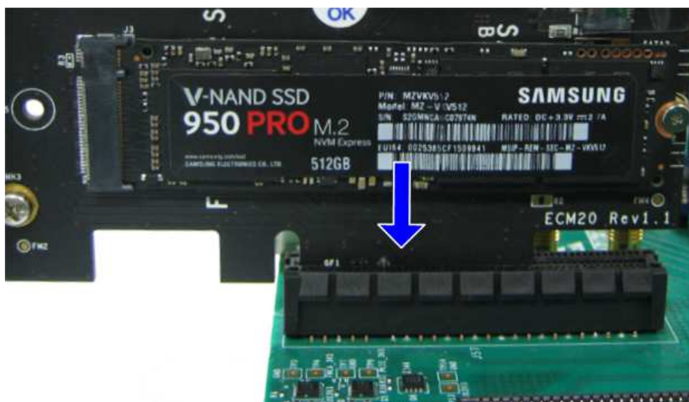
Figure 2-2 NVMe SSD connection on FPGA board
