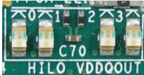
Figure 2-7 4-bit LED Status for user output
