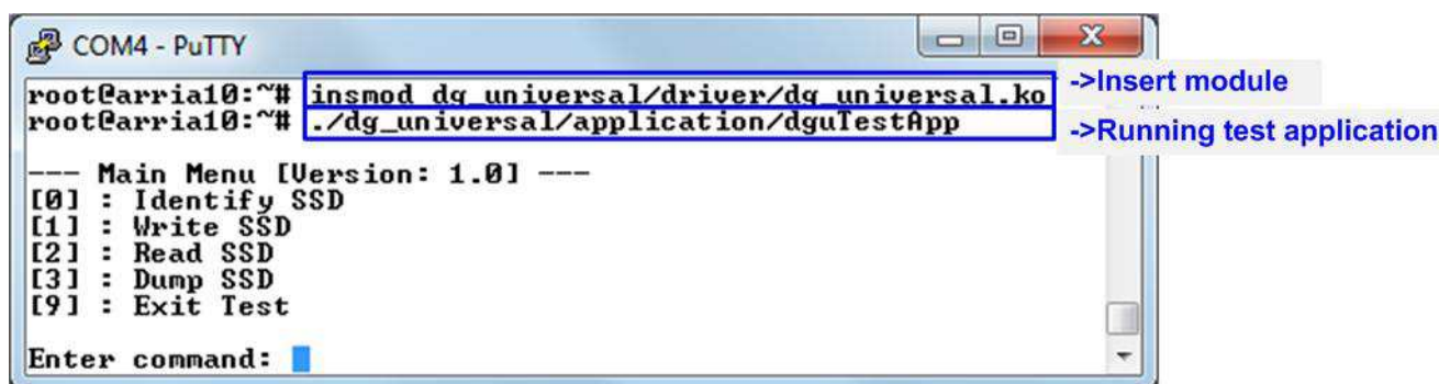
Figure 3-2 Insert module and running test application
