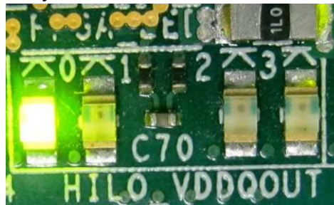
Figure 2-8 LED status after program configuration file and PCIe initialization complete
