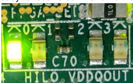
Figure 2-8 LED status after program configuration file and PCIe initialization complete
