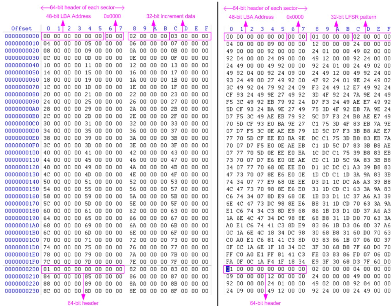
Figure 3-5 Example Test data in sector#0/#1 by increment/LFSR pattern
