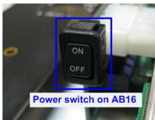
Figure 2-6 Power on AB16 board
