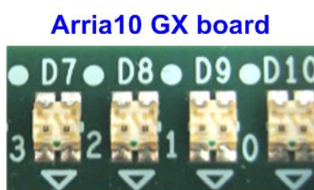
Figure 2-7 Four LEDs to show the current status
