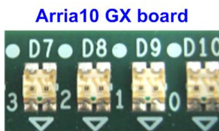
Figure 2-7 Four LEDs to show the current status
