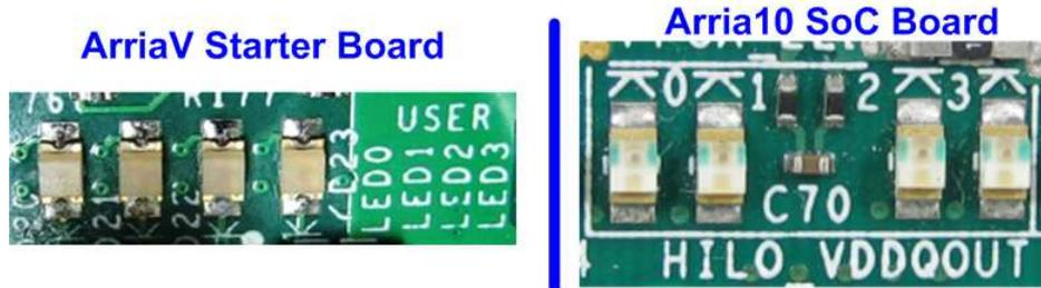
Figure 2-8 4-bit LED Status for user output
