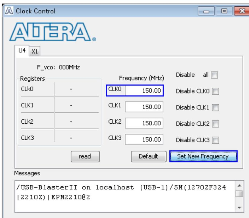
Figure 2-4 Set clock frequency for ArriaV GX board
