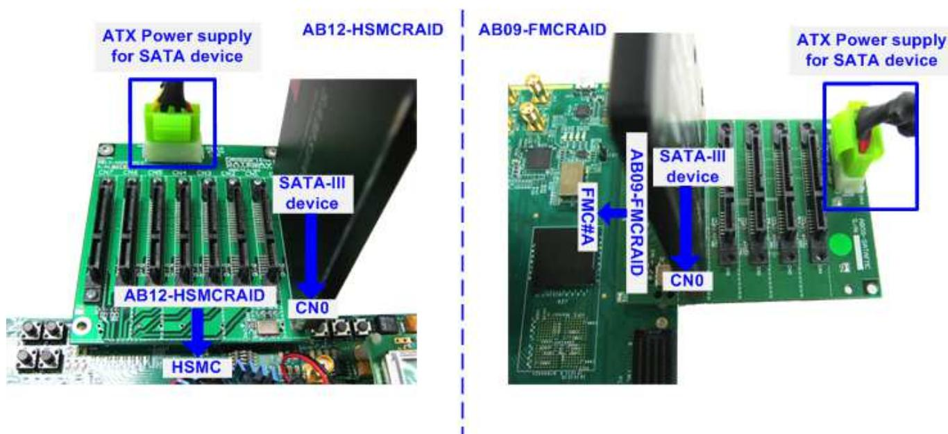
Figure 2-2 AB12 connection to FPGA board
