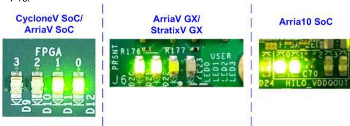
Figure 1-16 LED Status after setup complete
