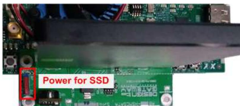
Figure 1-14 Power switch on HSMC adapter
