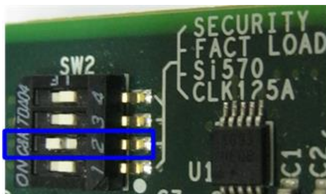
Figure 1-7 Set SW to enable Si570 for CycloneV SX SoC board
