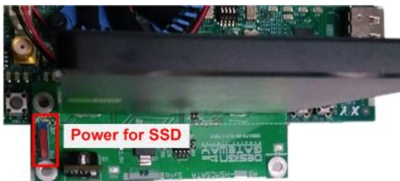
Figure 2-7 Power for SSD on HSMC adapter
