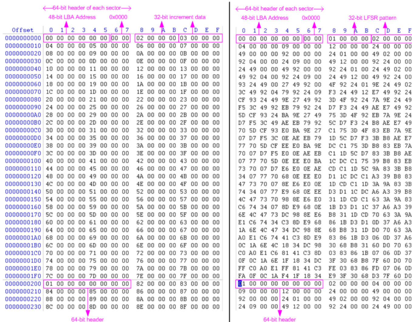
Figure 3-3 Example Test data in sector#0/#1 by increment/LFSR pattern
