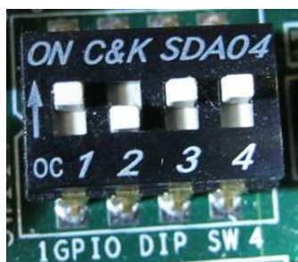
Figure 2-1 DIPSW setting for selecting auto-negotiation mode
