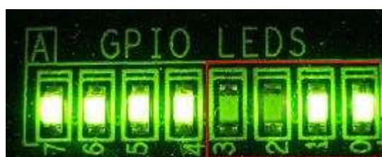
Figure 2-3 LED status after system set up complete on SATA-2 speed
