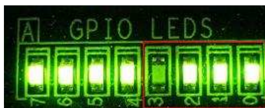
Figure 2-2 LED status after system set up complete on SATA-3 speed
