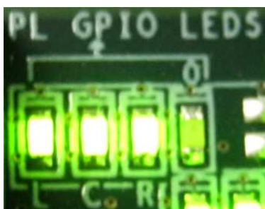
Figure 2-5 LED status after system set up complete on SATA-3 speed
