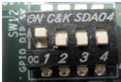
Figure 2-1 DIPSW setting for selecting auto-negotiation mode
