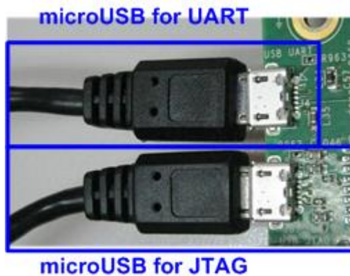
Figure 2-3 two micro USB cable connections on KCU105
