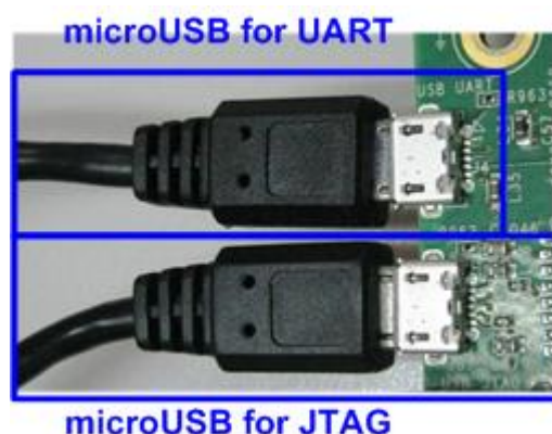
Figure 2-2 two micro USB cable connections on KCU105
