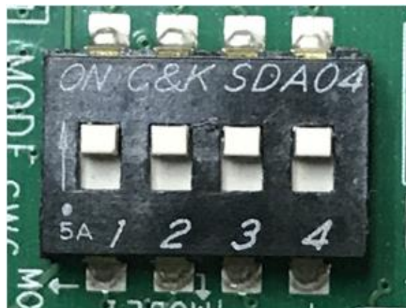
Figure 2-6 SW6 setting to configure PS from JTAG on ZCU102
