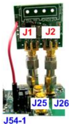
Figure 2-1 Connect CLKSMA board to AC701
