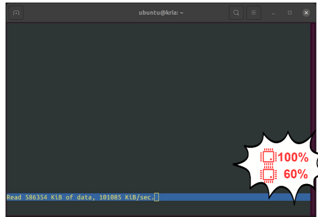
Figure 21 Example of Lynx UI downloading 1GB data via 1G Ethernet
