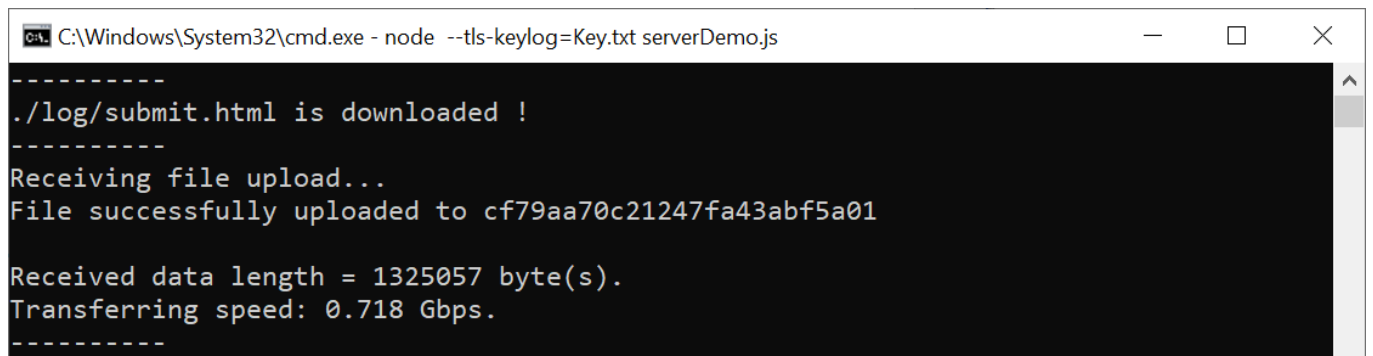
Figure 15 Server console when client upload data via submit.html page
