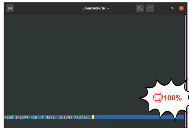
Figure 22 Example of Lynx UI downloading 1GB data via 10G Ethernet with hardware disabled
