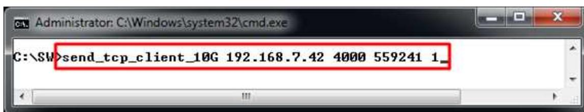
Figure 22 Command line for receiving demo on Verification mode
