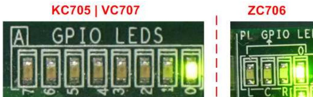
Figure 14 LED Status after push StartSW when DIPSW[1]=OFF
