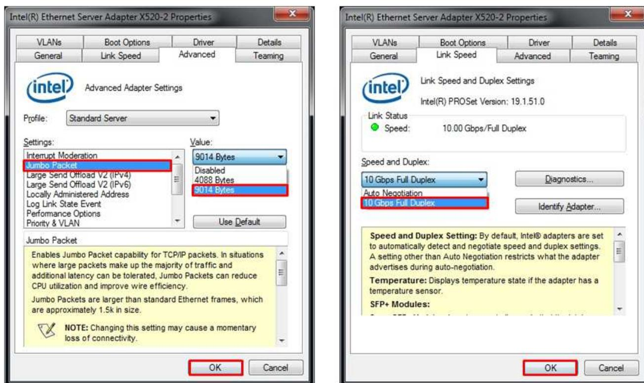
Figure 6 Link speed and Jumbo frame setup
