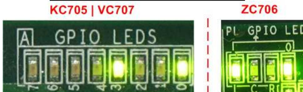
Figure 17 LED Status when running Sending Demo with Non-Jumbo frame
