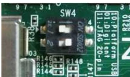
Figure 12 SW4 setting to use USB-to-JTAG on ZC706 board
