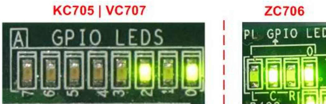
Figure 15 LED Status after push StartSW when DIPSW[1]=ON
