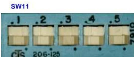
Figure 11 SW11 setting to configure PS from JTAG on ZC706 board
