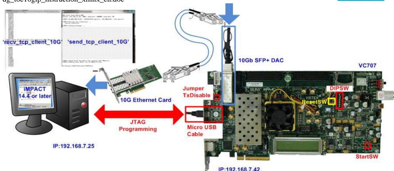
Figure 2 TOE10G-IP Demo Environment Setup on VC707
