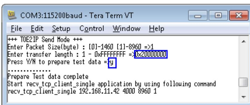
Figure 18 Input menu with test pattern selection (transfer length <= 512 Mbyte)
