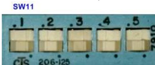
Figure 4 SW11 setting to configure PS from JTAG on ZC706 board
