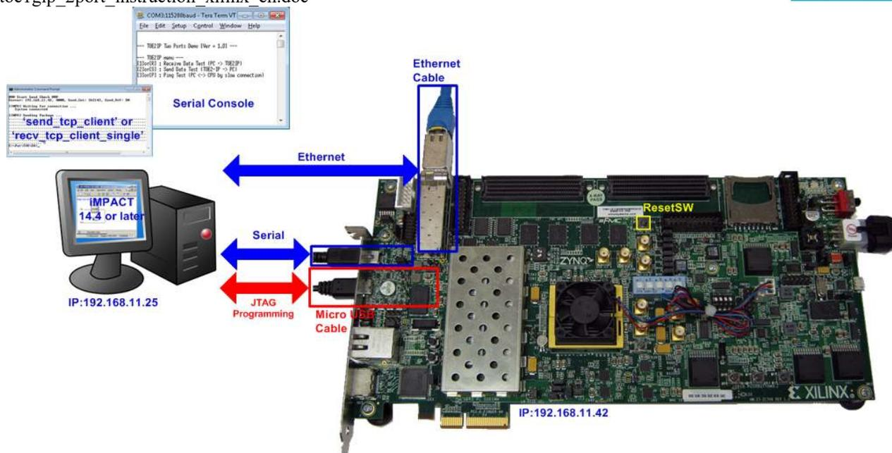
Figure 2 TOE1G-IP Two-Port Demo Environment Setup on ZC706
