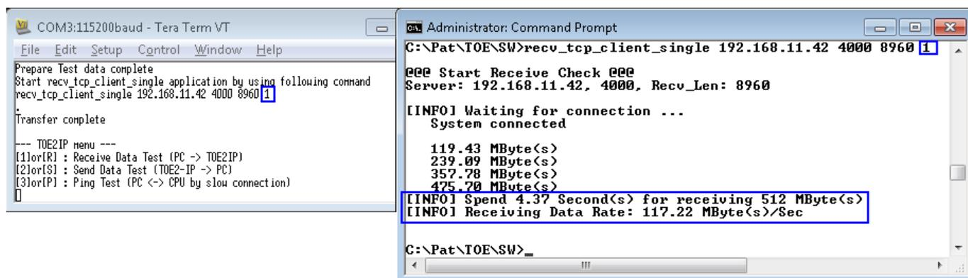
Figure 23 Test Result when enable data verification
