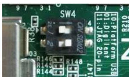
Figure 5 SW4 setting to use USB-to-JTAG on ZC706 board
