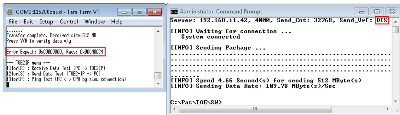
Figure 16 Error message on Serial console when data verification fail
