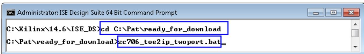
Figure 7 Example command script for download to ZC706 by ISE tool
