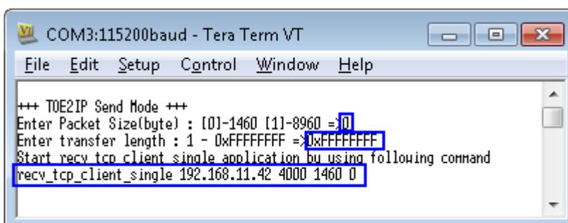
Figure 17 Input menu without test pattern selection (transfer length > 512 Mbyte)
