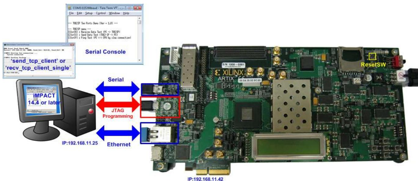
Figure 3 TOE1G-IP Two-Port Demo Environment Setup on AC701
