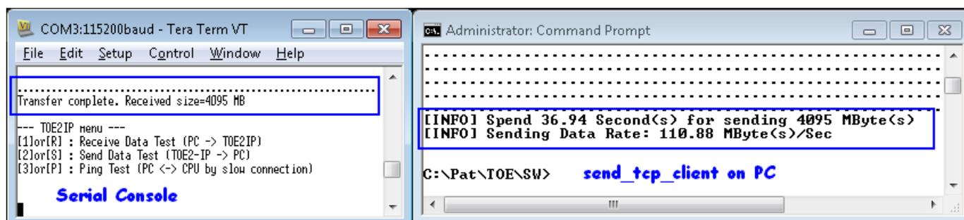
Figure 13 Test Result when transfer size is more than 512 MB
