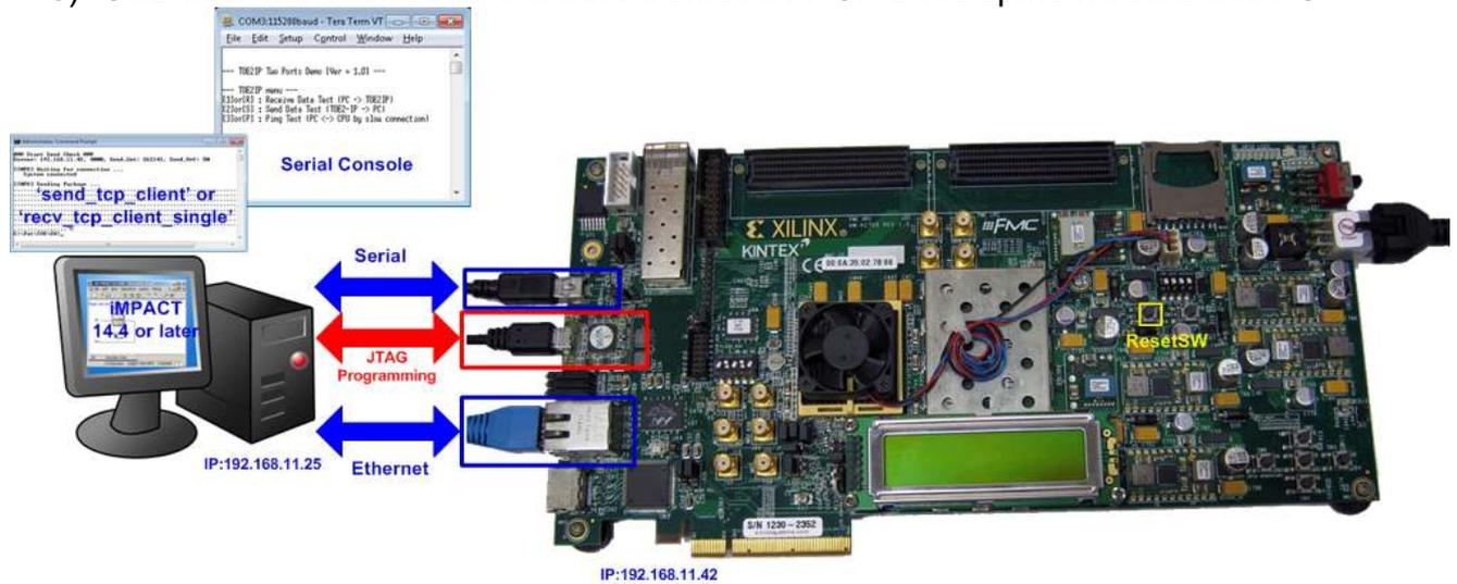
Figure 1 TOE1G-IP Two-Port Demo Environment Setup on KC705
