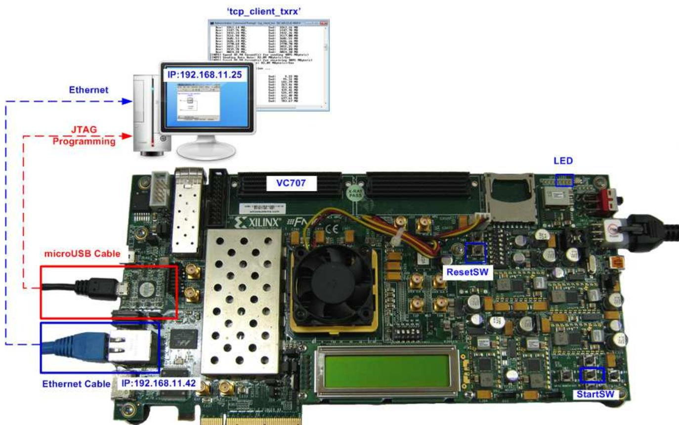
Figure 1-3 TOE1G-IP Full Duplex Demo Environment Setup on VC707
