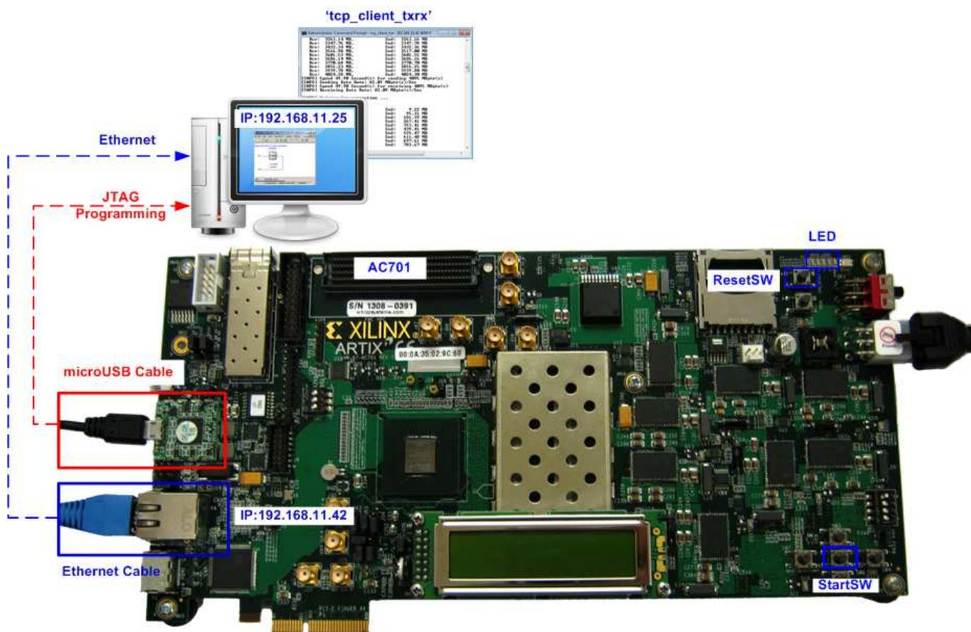
Figure 1-1 TOE1G-IP Full Duplex Demo Environment Setup on AC701
