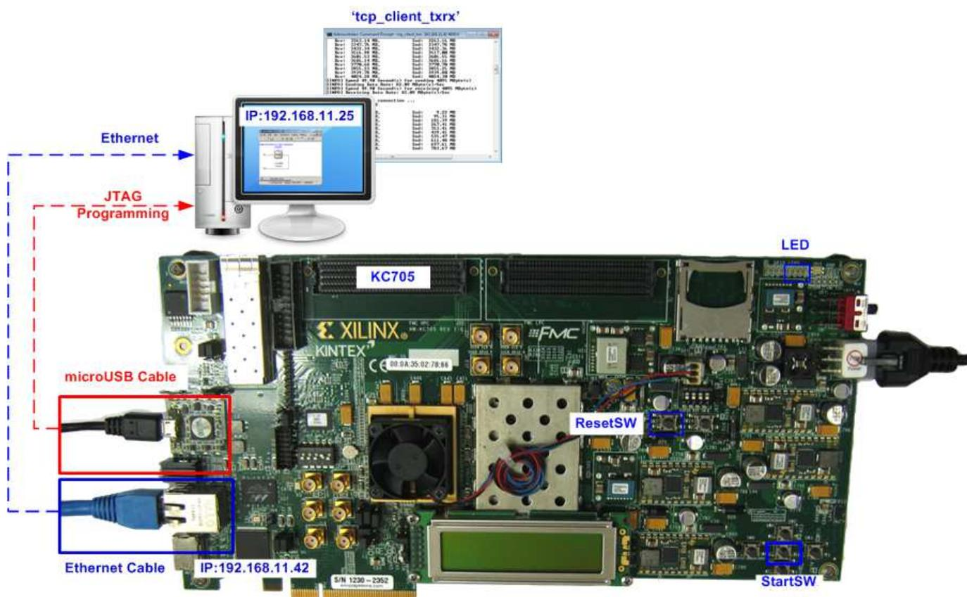
Figure 1-2 TOE1G-IP Full Duplex Demo Environment Setup on KC705
