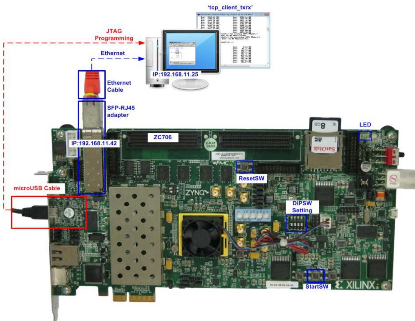
Figure 1-4 TOE1G-IP Full Duplex Demo Environment Setup on ZC706
