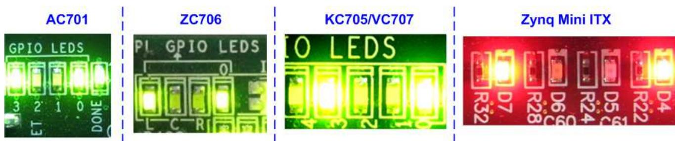
Figure 4-4 LED Status when running full duplex Demo in both modes
