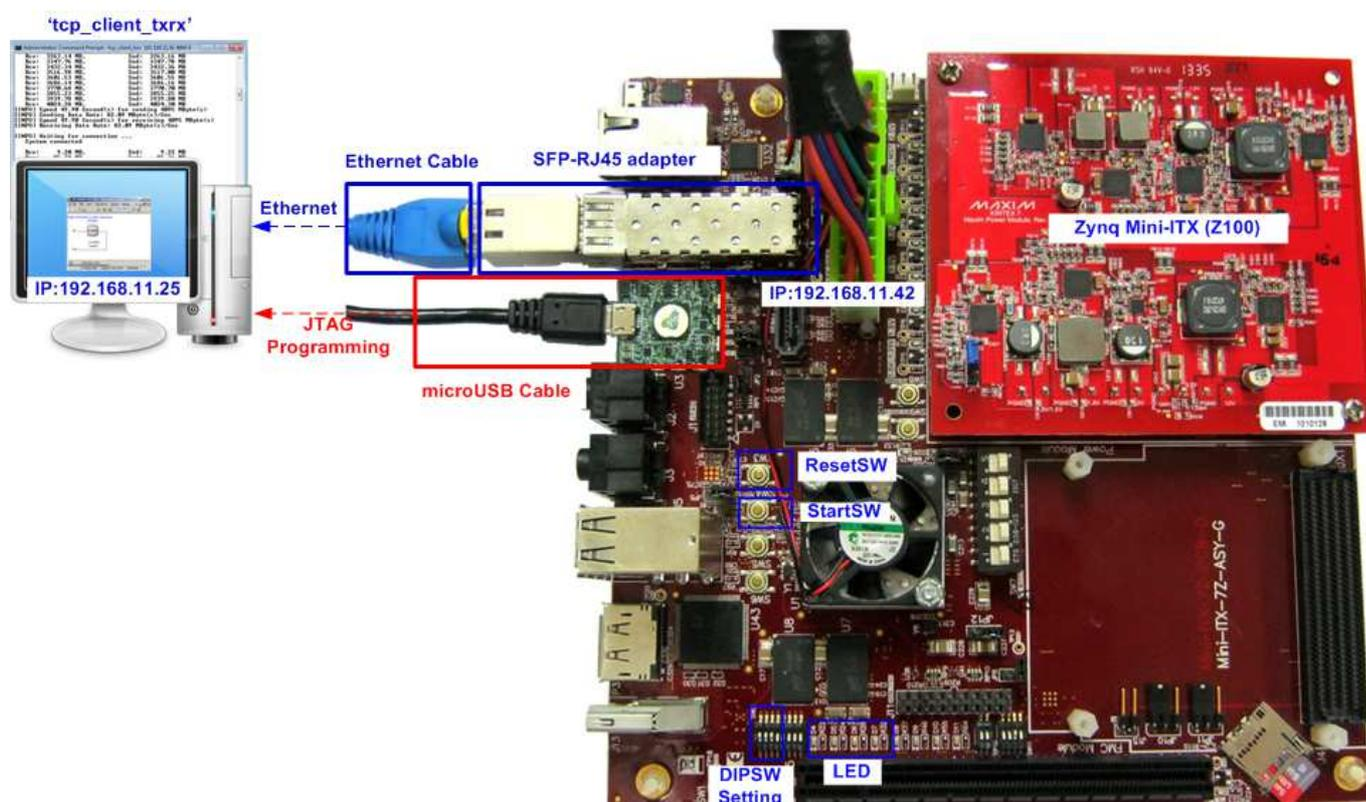
Figure 1-5 TOE1G-IP Full Duplex Demo Environment Setup on Zynq Mini-ITX (Z100)
