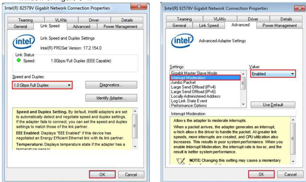
Figure 3-4 Link speed and Jumbo frame setup
