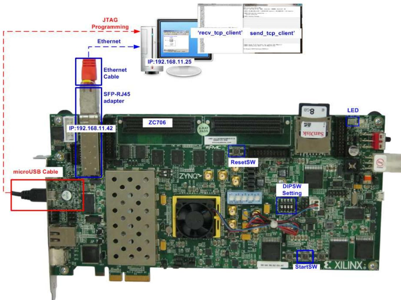
Figure 1-4 TOE1G-IP Demo Environment Setup on ZC706
