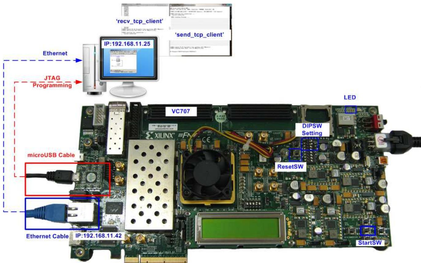
Figure 1-3 TOE1G-IP Demo Environment Setup on VC707
