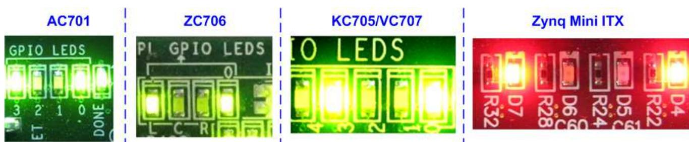
Figure 4-11 LED Status when running Sending Demo with Non-Jumbo frame
