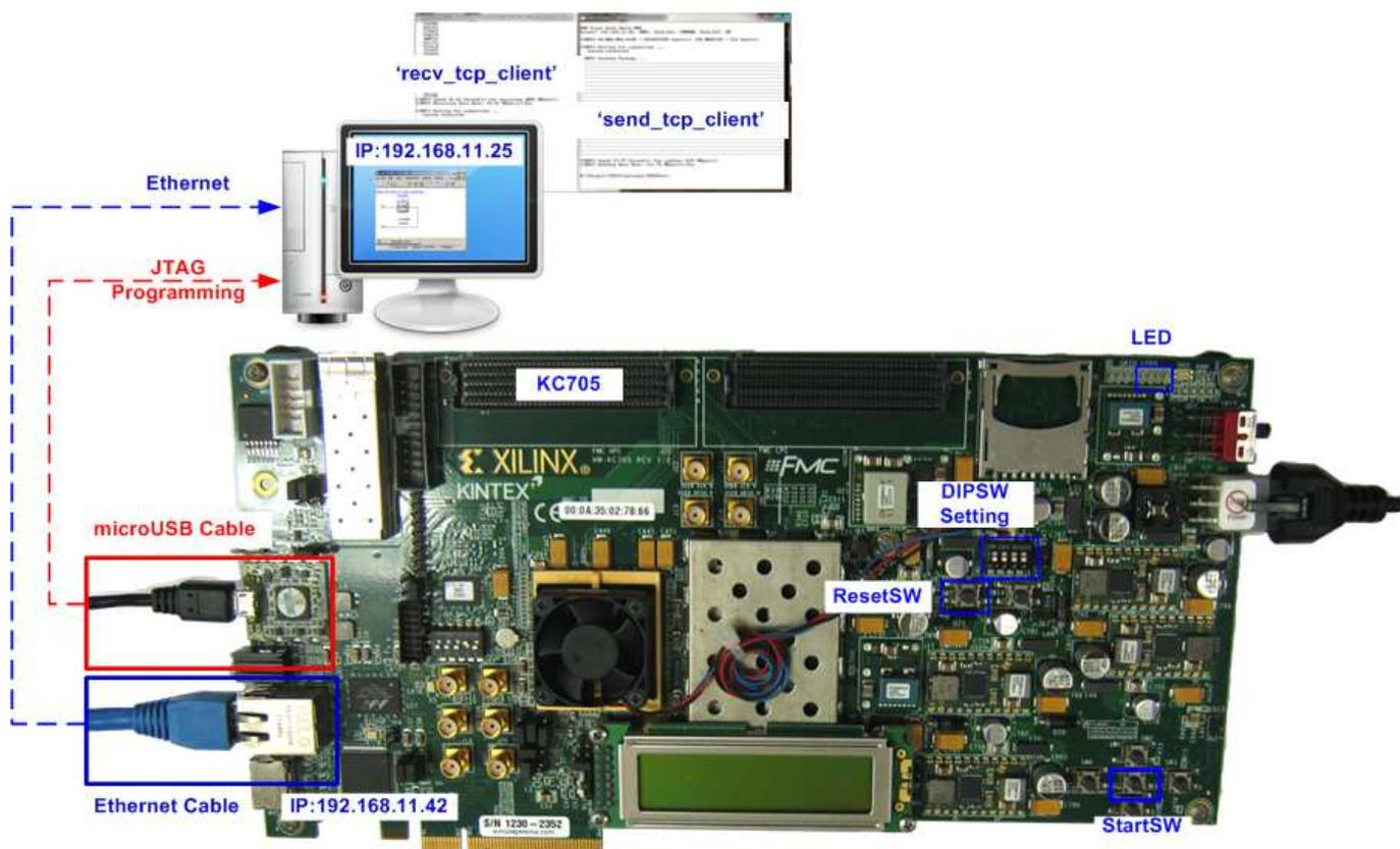
Figure 1-2 TOE1G-IP Demo Environment Setup on KC705
