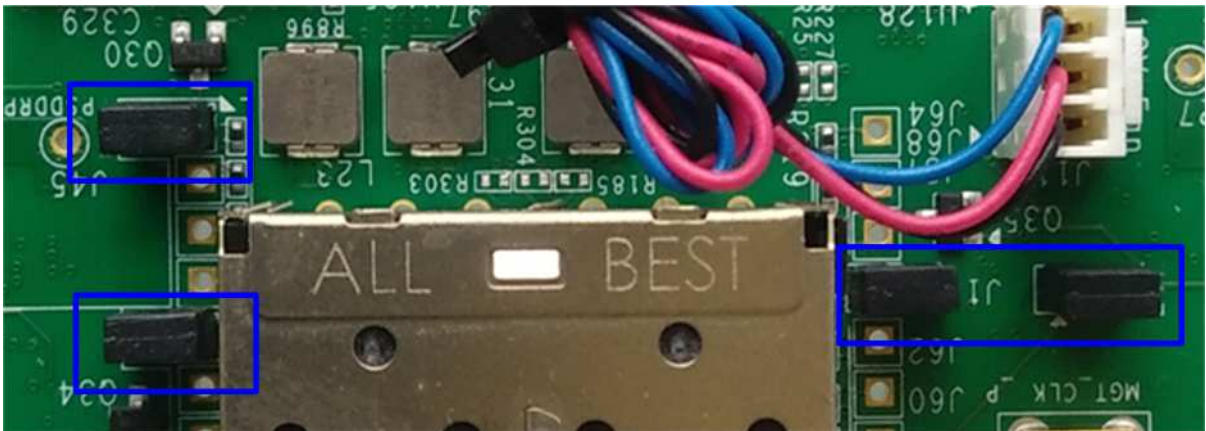
Figure 4-2 Set SFP[0]-[3] TX DISABLE for ZCU102
