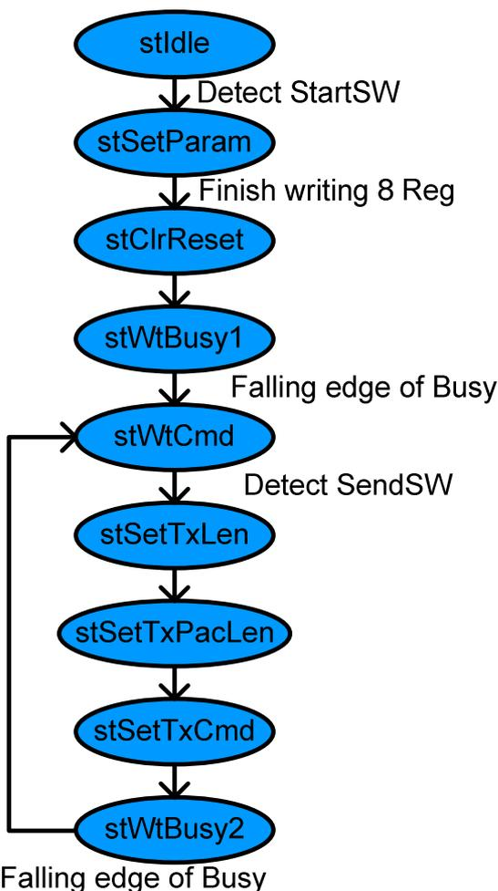
Figure 5 State Machine Diagram within User Module
