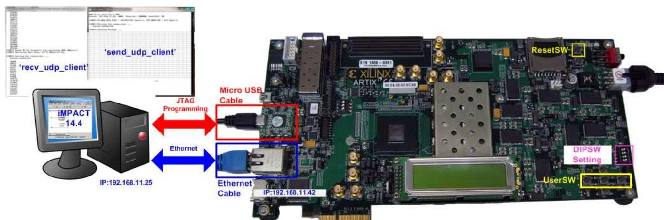
Figure 2 UDPIP Demo on Development board
