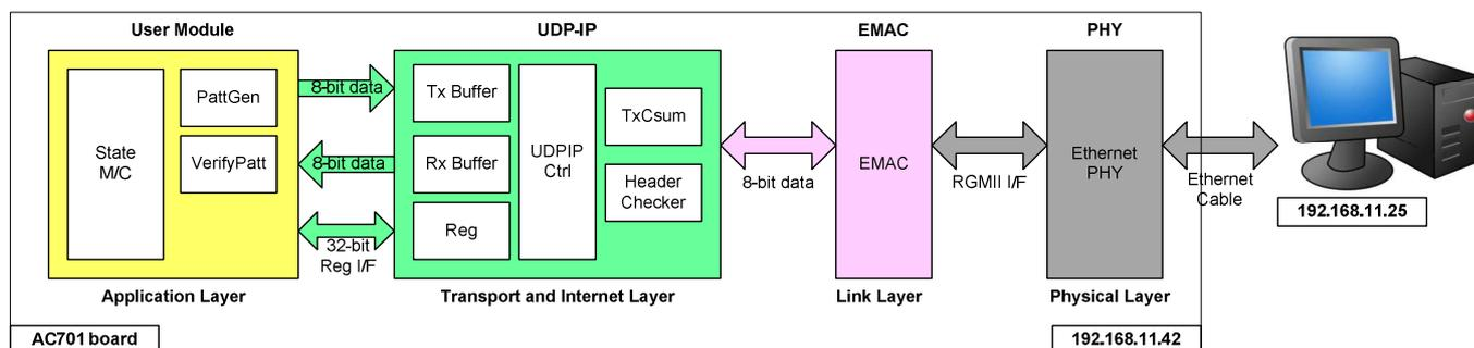
**Figure 3 Hardware Architecture in AC701 reference design**
