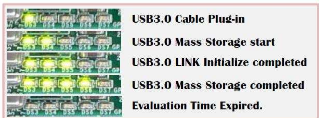
Figure 17: USB3.0 device operation LED status on SP605 board
