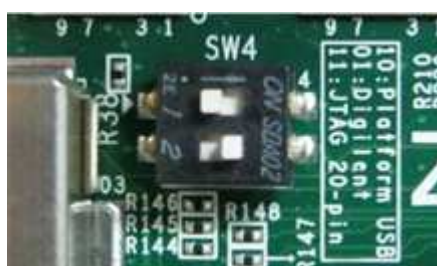
Figure 16: SW4 setting on ZC706 board
