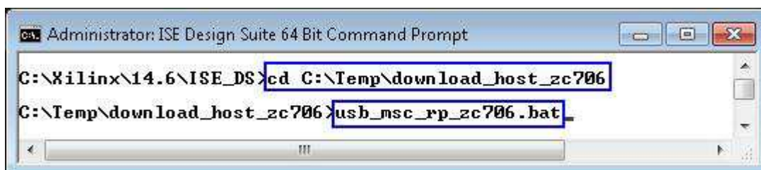
Figure 17: Run bat file to program bit and elf file on ZC706 board
