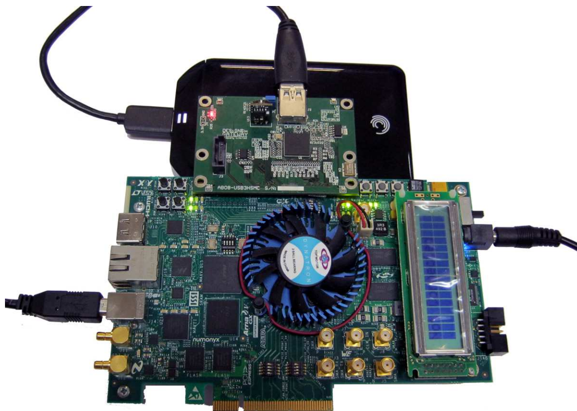
Figure 5: Adapter board connection to ArriaV GX starter board
