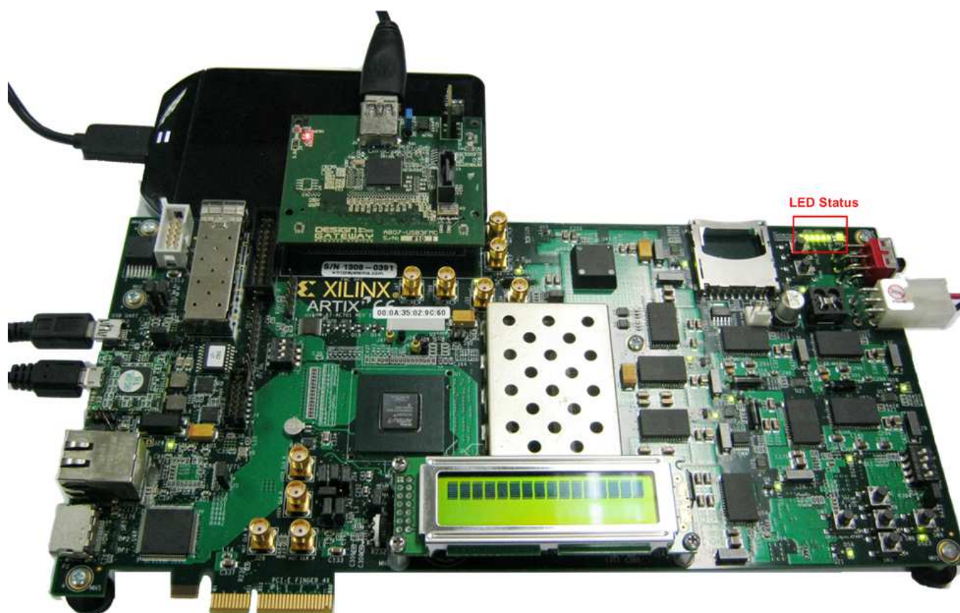
Figure 13: Adapter board connection to AC701
