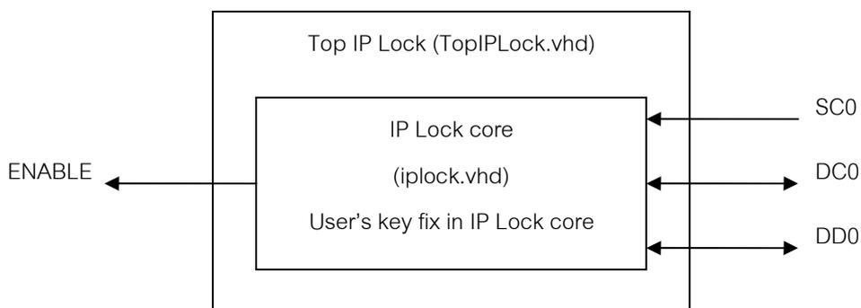
Figure 3-2 Top level of IP Lock for Altera FPGA
