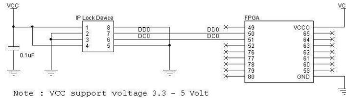
Figure 4-8 Typical circuit of IP Lock device
