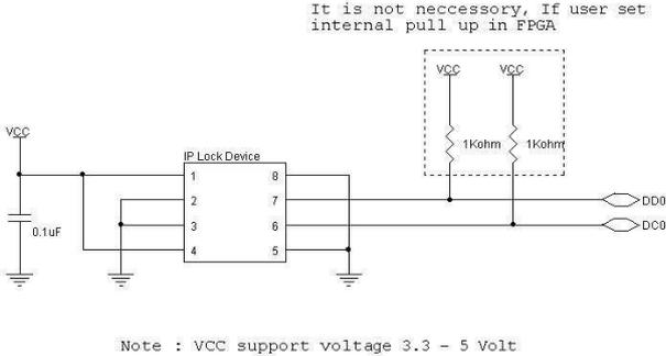
Figure 4-1 Schematic of IP Lock Device
