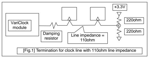
Value of the termination resistor should be determined so that output current value of VariClock will not exceed the maximum output current of +24mA/-24mA. Each of 220ohm pull-up and pull-down Thevenin resistors is implemented in the figure1 for clock line with 110ohm line impedance. In this case, even the damping resistor value is 0ohm, VariClock can drive the clock signal to High or Low level because its drive current is 3.3[V] / 220[ohm] = 15mA as allowable range as below 24mA.
