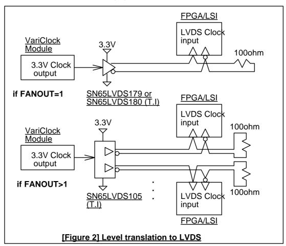
When clock should be supplied to only one device (FANOUT=1), user can use single channel translator such as SN65LVDS179 or SN65LVDS180 from Texas-Instruments. If more than two devices require LVDS clock input (FANOUT>1), it is recommendable to use clock driver that can translate 3.3V-LVTTL to LVDS and also can increase clock channel such as SN65LVDS105 from Texas-Instruments
