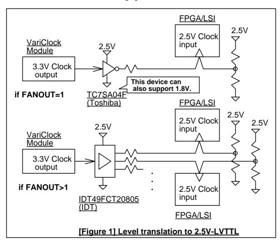
When clock should be supplied to only one device (FANOUT=1), single level translation of one-input to one-output is enough. In this case high-speed one-gate logic such as TC7SA04F from Toshiba is suitable because of the board area. Though the output clock phase shifts 180 degree from input clock because of the inverter buffer, it is not the problem unless direct clock output from VariClock is supplied to another part of the circuit. This TC7SA04F also supports 1.8V power supply voltage.
