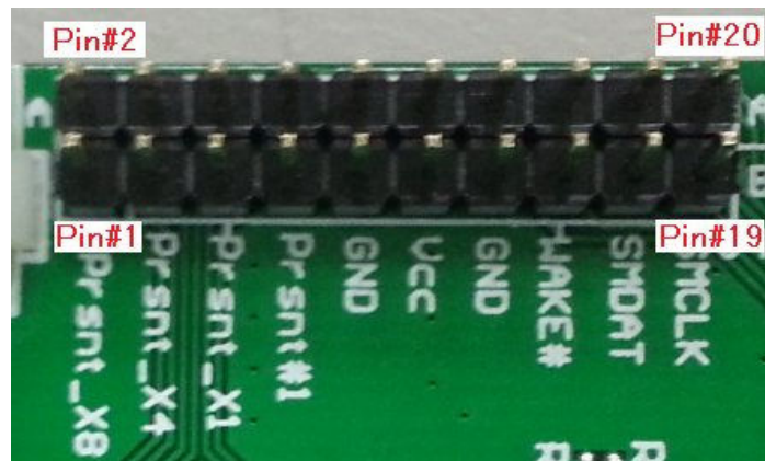
Figure-5: J4 pin header for PCIe side-band signal
