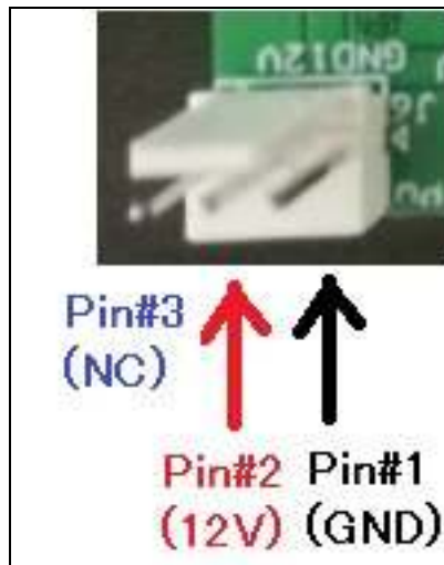
Figure-5: J6 connector for fan power supply
