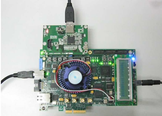
Evaluation on Cyclone® IV GX FPGA Dev. kit with AB08-USB3HSMC
