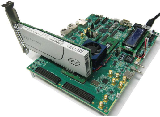
Evaluation on Intel® Arria® 10 SX FPGA Development Kit with Intel® NVMe PCIe SSD
