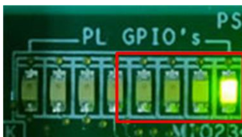
Figure 2-5 LED status after programming configuration file and finishing PCIe initialization
