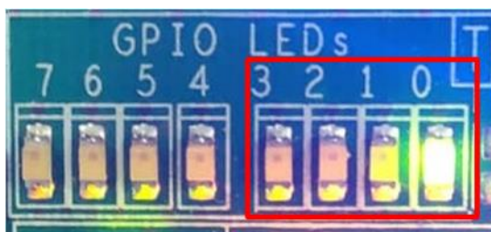
Figure 2-8 LED status after programming configuration file and finishing PCIe initialization
