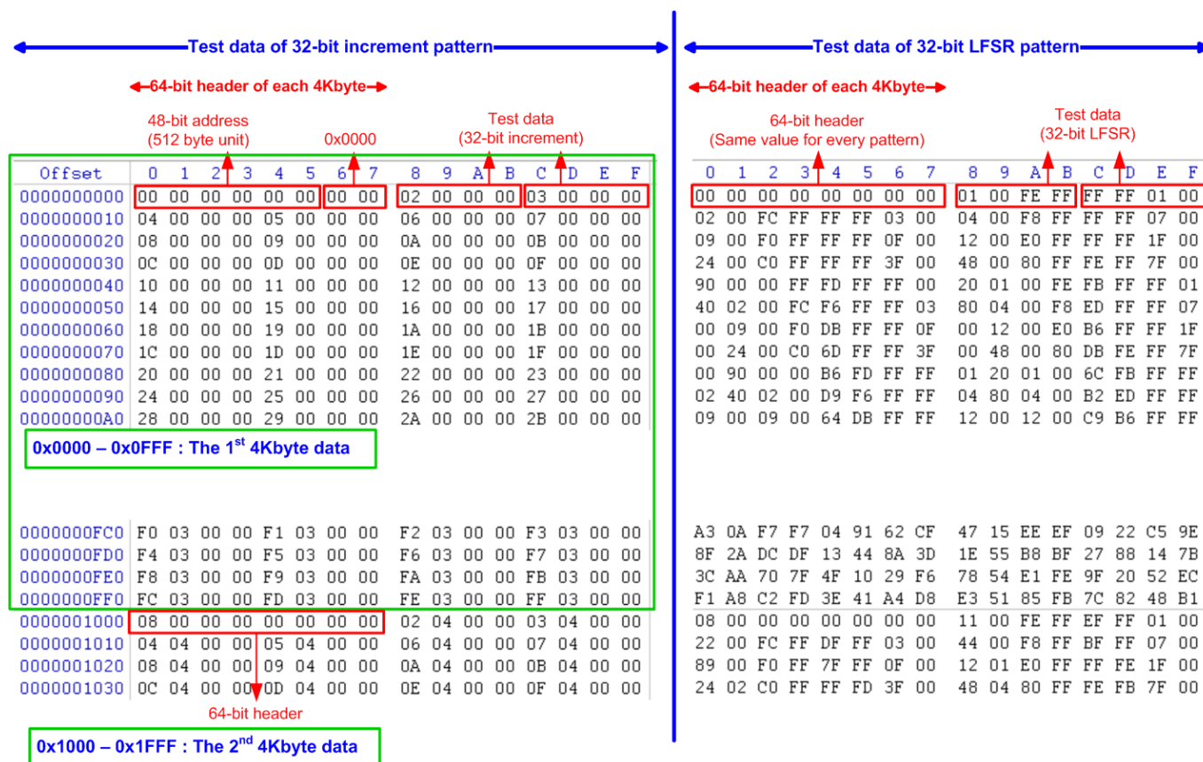
Figure 2-4 Example Test data of the 1st and 2nd 4Kbyte data by using incremental/LFSR pattern
