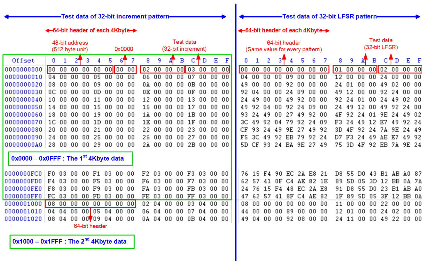
Figure 2-5 Example Test data of the 1 st and 2 nd 4Kbyte data by using incremental/LFSR pattern
