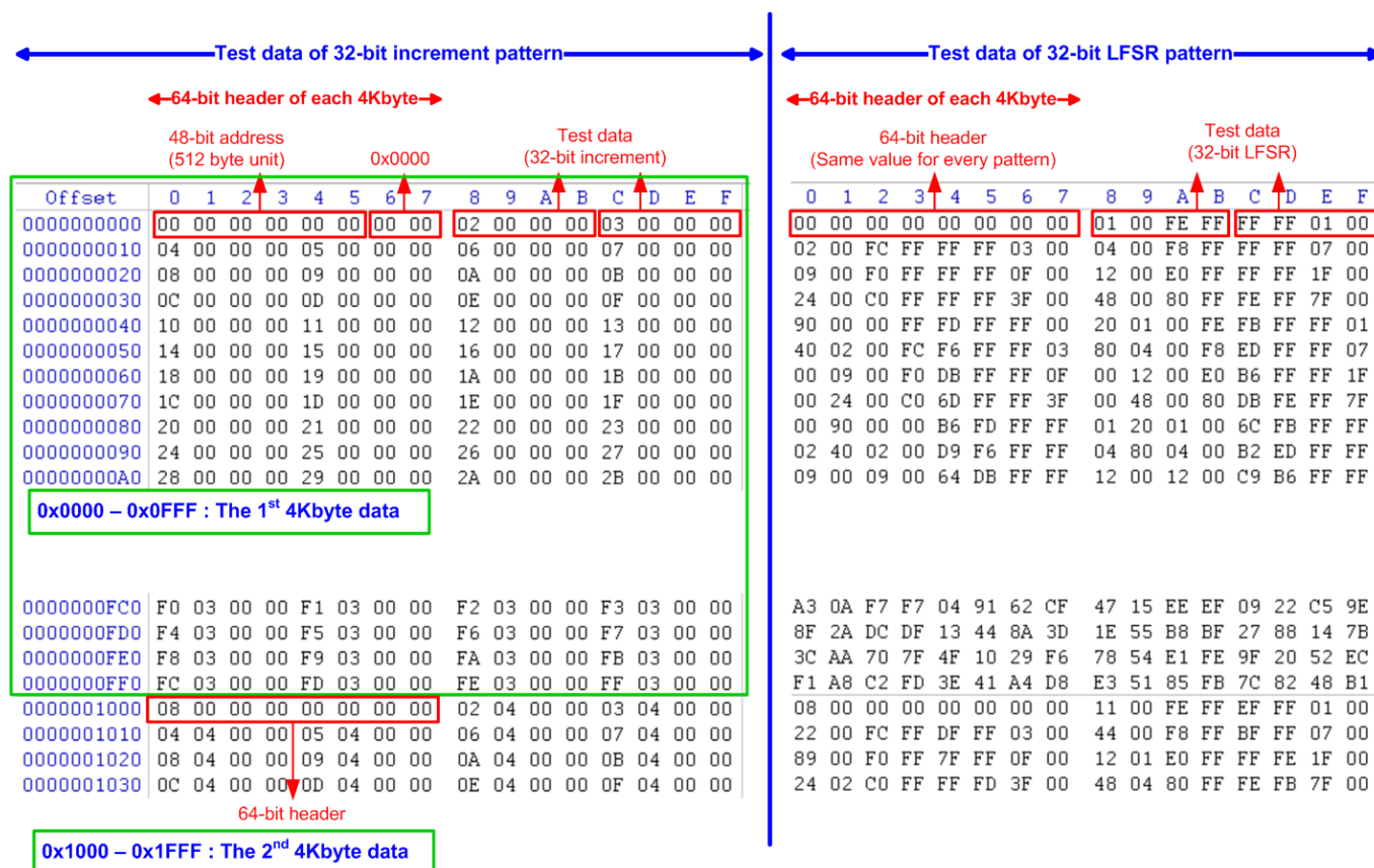
Figure 2-5 Example Test data of the 1 st and 2 nd 4Kbyte data by using incremental/LFSR pattern
