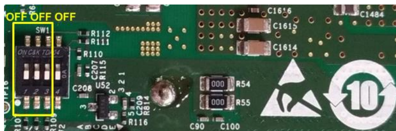
Figure 2-3 SW1 setting on Agilex F-series board
