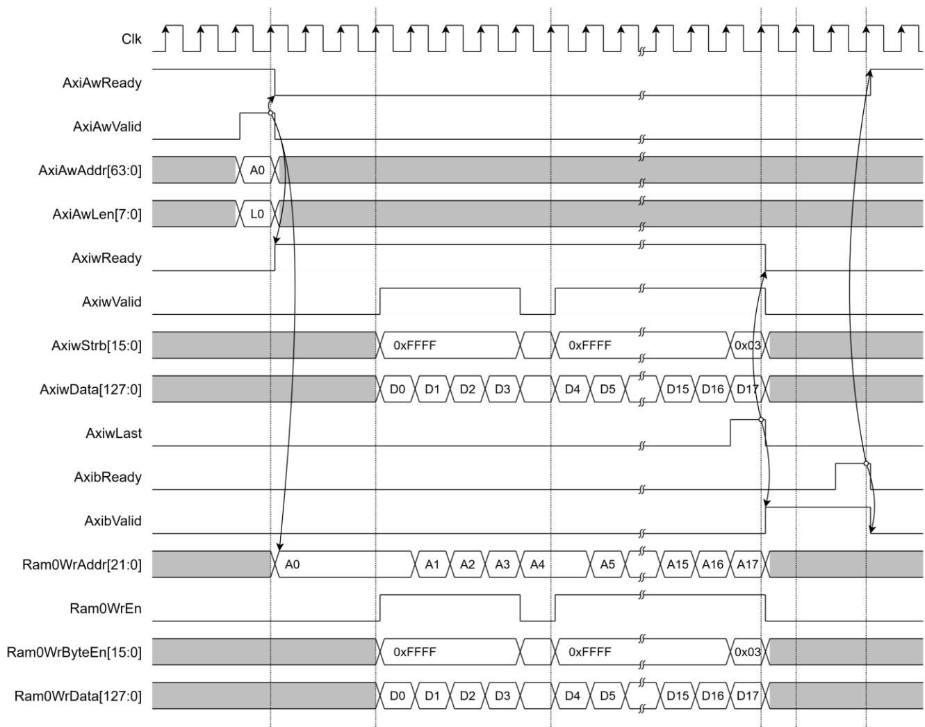
Figure 5 Example timing diagram of writing data to RxRam via AXI bridge
