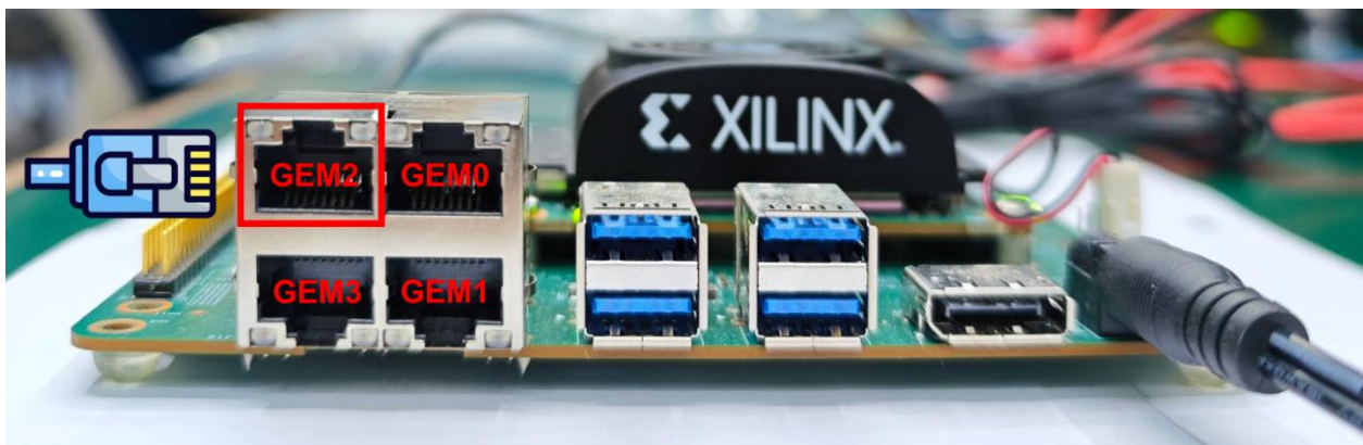
Figure 2 RJ45 GEM2 connector location on the KR260 board
