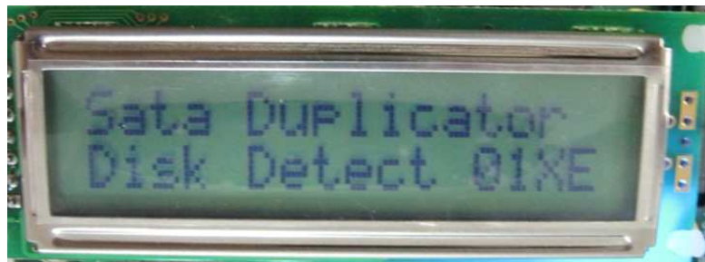
Figure 2-8 LCD Text Display when Disk not available or error.
