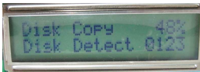
Figure 3-4 Disk Copy Progress Status on LCD
