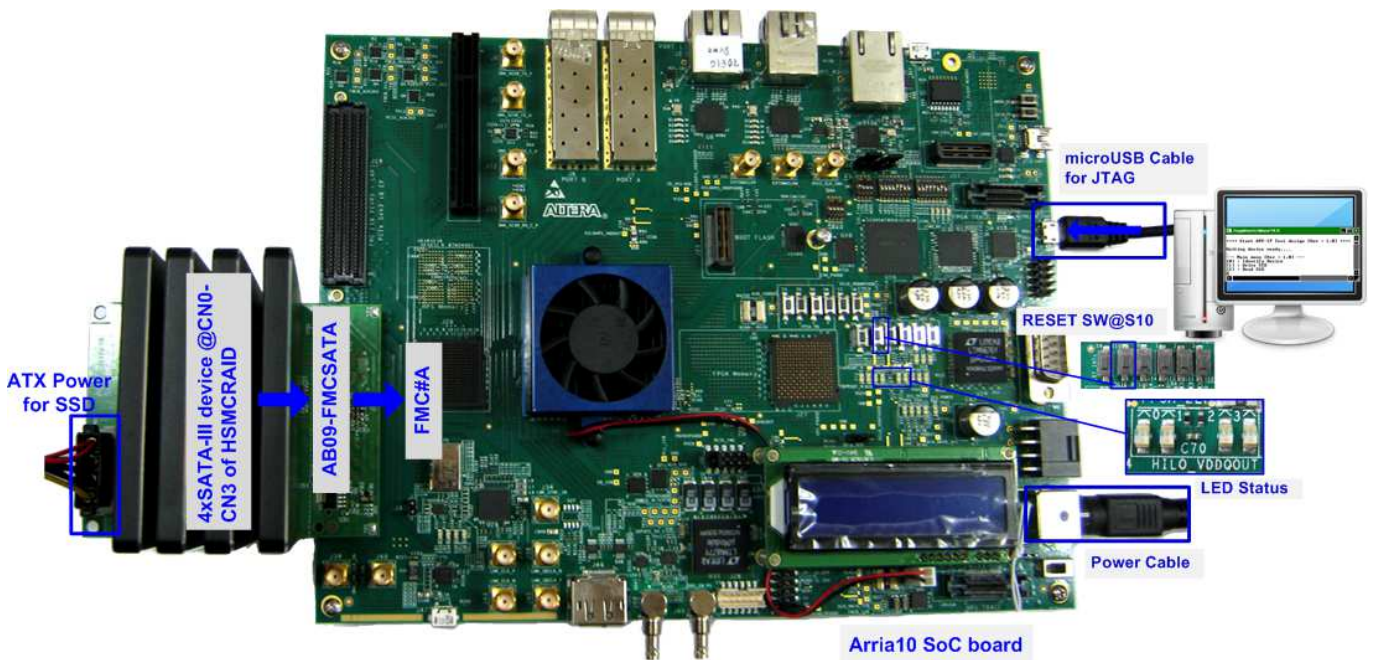
Figure 1-2 SATA Host RAID0 Demo Environment Setup on Arria10 SoC Development Board
