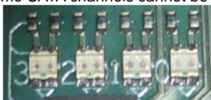
Figure 7 LED Status when all SATA devices LINKUP and system is in Idle
