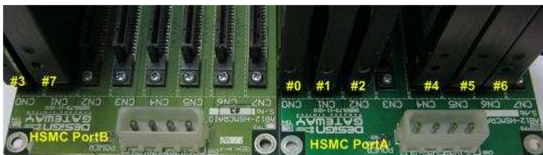
Figure 4 SATA-III device connection on two HSMCRAID boards
