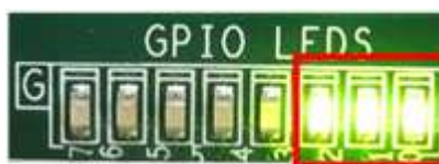
Figure 6 LED status after system set up complete when linkup at SATA-3 speed
