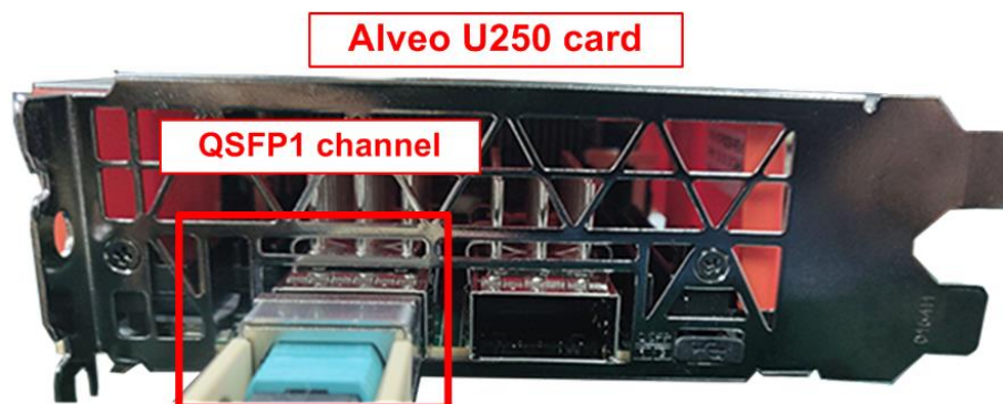
Figure 3-2 100Gb connection on Alveo card by QSFP28 transceiver and MPO to MPO cable
